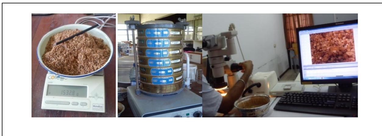
Figure 2 - Weighing, dry sieving, and microscopic analysis.
